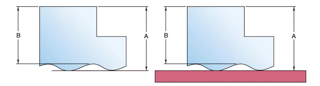
When measured at location A, the part seems to be within tolerance; however, measuring at location B creates a problem because the measurement is being taken at a high spot of the surface roughness, which may make the part appear to be unacceptably out of tolerance.
