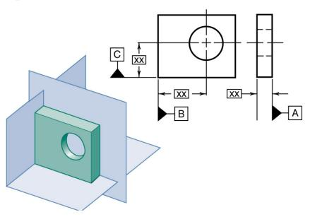
The most useful secondary datum feature can be a hole that is perpendicular to the primary datum. The surface creates the primary datum, and the hole creates two perpendicular planes.
