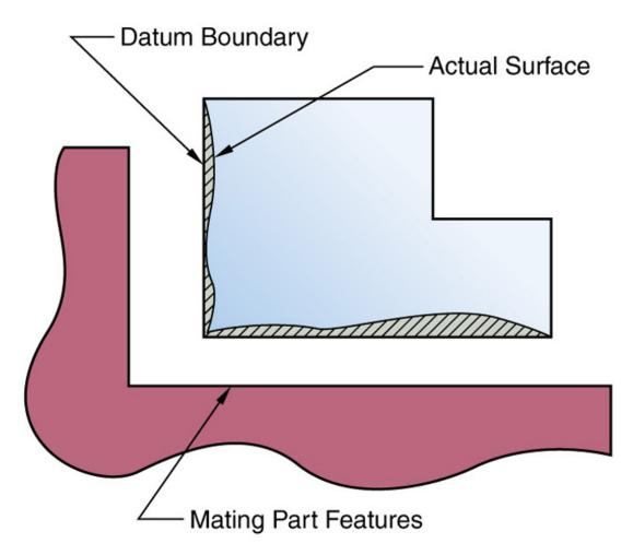
However, it may be acceptable for the surfaces to have depressions, which will not interfere with the mating of the parts.
