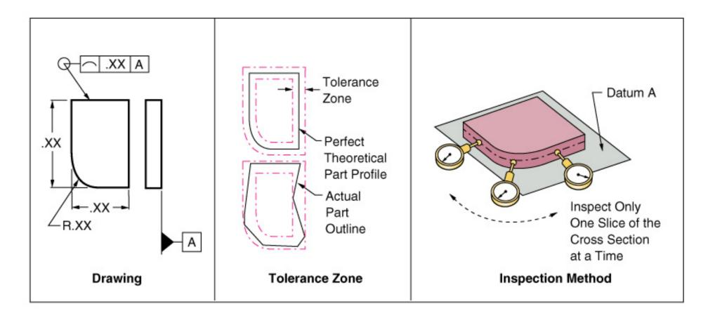
Profile is usually used to control shapes that are combinations of contiguous straight lines, circular arcs, and other curves.
