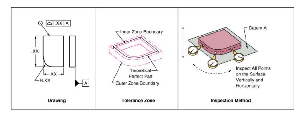
In line profile control we have to inspect only one slice along the edge – horizontally, but in surface profile control we inspect different slices – all points both horizontally and vertically.
