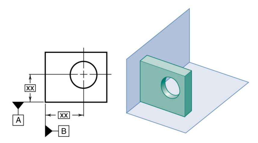
These features should be machined first. All dimensions should be shown from these surfaces.
