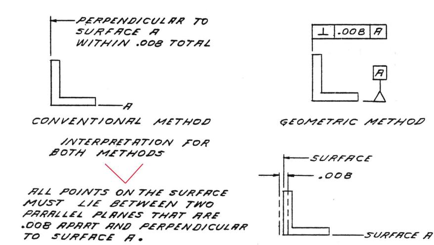
All dimensions and tolerances that are shown on a print must be maintained.
