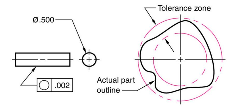
If the roundness control were removed, the shaft would still have to be round within the limits of the diameter tolerance, per Rule 1.
