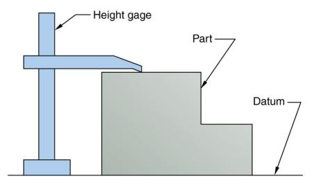
These datum features are clearly marked in the drawings to indicate which are the reference surfaces to make measurements from.
