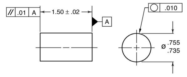
The left example defines the parallelism between two surfaces, the right one shows the circularity.
