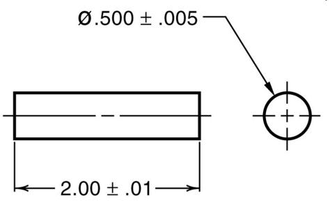
In this case the circularity control is the equivalent of 0.005.
