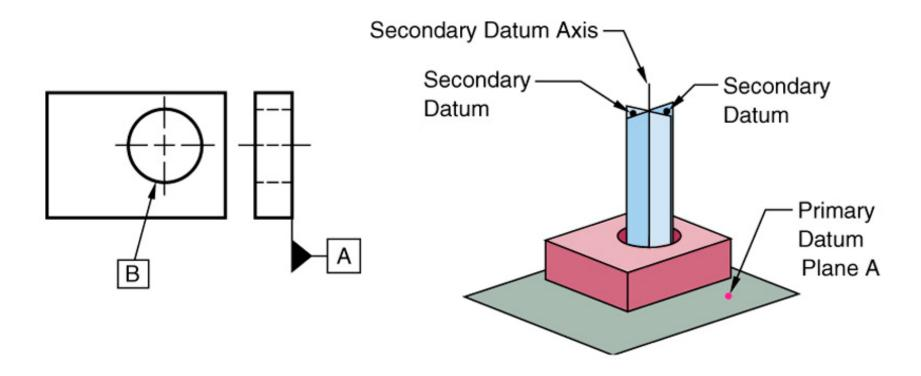
This reference frame is the most commonly used and is called the *plane and cylinder reference frame*. Here the primary datum plane is identified with the letter A, and secondary cylinder surface is identified with the letter B.
