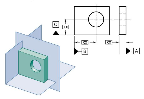
The critical part of datum selection is identification of the **primary datum**. In many cases, this will be the only datum, and it has to be chosen based on a number of criteria:
