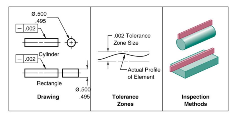
• Axis straightness. This compares the axis of a cylindrical feature to a perfectly straight line.
