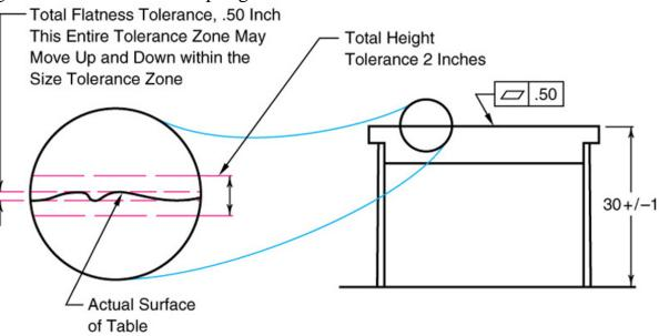
*Size tolerances* alone are sometimes not enough to meet the design needs of a part. *Relationships between features* may also need to be controlled.
