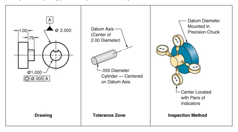
• **Runout**. There are two types of runout: single circular element (slice) and total (cylinder).
