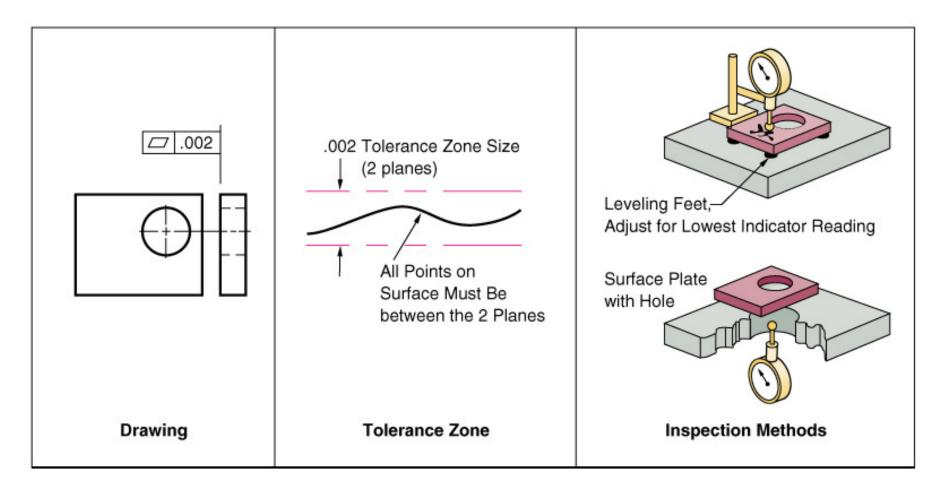
That is, the surface is compared to a perfect plane (straightness applied in all directions).
