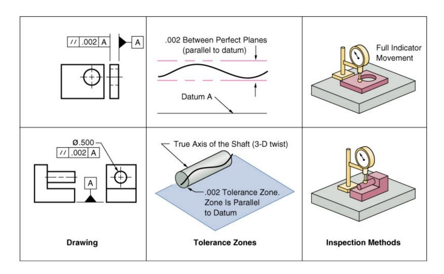
• **Perpendicularity**. This could be considered flatness or straightness of an axis 90 degrees to a datum.
