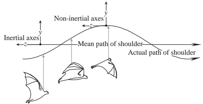
Fig. 2. Orientations of and relationships between the inertial and non-inertial coordinate systems; the actual and mean paths of the shoulder are depicted from a lateral view of the bat moving from left to right across the figure. The  $x$  axis is perpendicular to the plane of the page and is represented by the filled circles.
