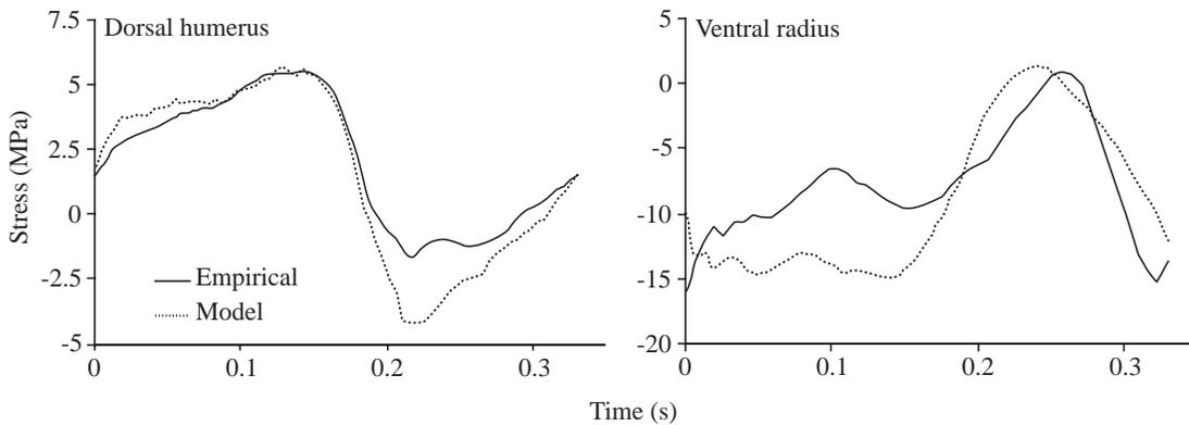
Fig. 14. Comparison of transversely oriented bone stresses computed from the model, assuming the spanwise elastic modulus of the skin  $E_{xx}$  to be 0.5 MPa, with the forces calculated from empirically gathered rosette strain data and the published value for the Poisson's ratio of bone.
