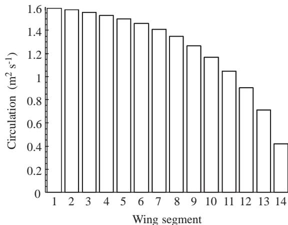
Fig. 4. Elliptical distribution of the magnitude of aerodynamic forces at each wing segment; segment 1 is adjacent to the shoulder and segment 14 includes the wingtip (see Fig. 1).
