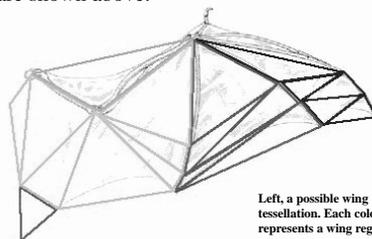
Left, a possible wing tessellation. Each color represents a wing region which is further broken down to triangles.
