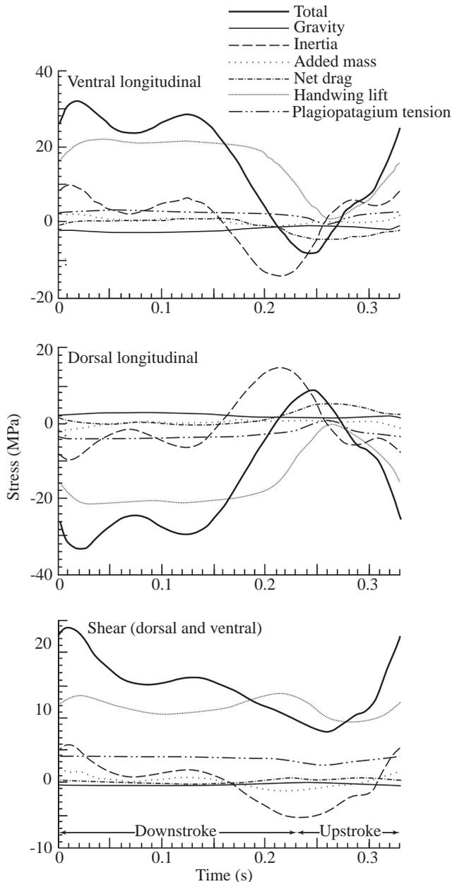
Fig. 11. Longitudinal and shear stresses at the radial midshaft computed by the model for an entire wingbeat assuming the spanwise elastic modulus of the skin  $E_{xx}$  to be 0.5 MPa; total stress (solid heavy line) is partitioned into components due to each of the individually modeled forces exerted on the wing.
