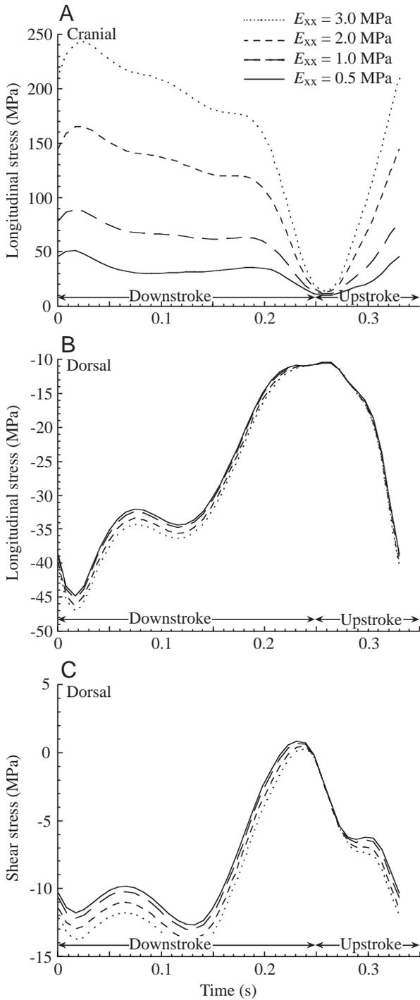
Fig. 8. Longitudinal and shear stresses computed by the model at the midshaft of the humerus throughout the wingbeat cycle as a function of spanwise elastic modulus of the skin,  $E_{xx}$ . (A) Longitudinal stresses on the cranial surface of the bone. (B) Longitudinal stresses on the dorsal surfaces of the bone. (C) Shear stresses on the dorsal surface of the bone.
