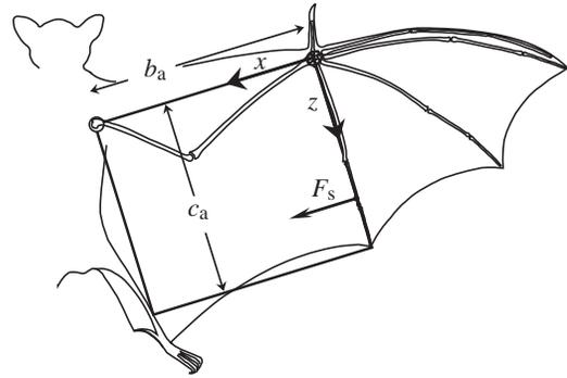
Fig. 5. Schematic diagram of the rectangular idealization of the armwing membrane. The  $x$  and  $z$  coordinate axes used to describe membrane deflection mathematically are indicated; the  $y$  axis is perpendicular to the plane of the membrane.  $F_s$  indicates the point of application and approximate orientation of the skin internal force,  $c_a$  is the mean armwing chord and  $b_a$  is the instantaneous shoulder-to-carpus distance.
