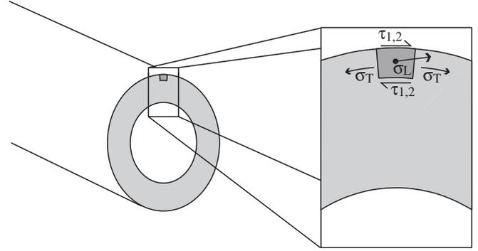
Fig. 7. Definitions of the orientations and signs of longitudinal and shear stresses with respect to midshaft cross sections of the humerus and radius.  $\tau_{1,2}$ , shear stress;  $\sigma_L$ , longitudinal stress;  $\sigma_T$ , transverse stress.
