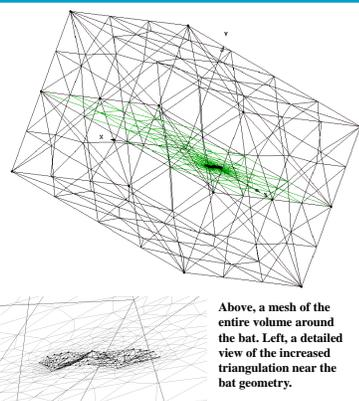
Above, a mesh of the entire volume around the bat. Left, a detailed view of the increased triangulation near the bat geometry.
