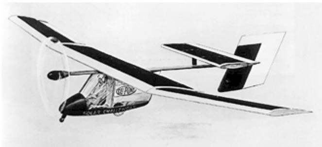
Using in-house computer programs, AeroVironment engineers Peter Lissaman and Bart Hibbs designed the unusual wings and stabilizers, which they made flat on top to hold the solar cells. Hibbs developed the aerodynamic design for the propeller with another in-house computer program. The result was a "smooth and docile" aircraft that dropped in a steady, wing-level attitude when stalled and rapidly regained unstalled flight.
