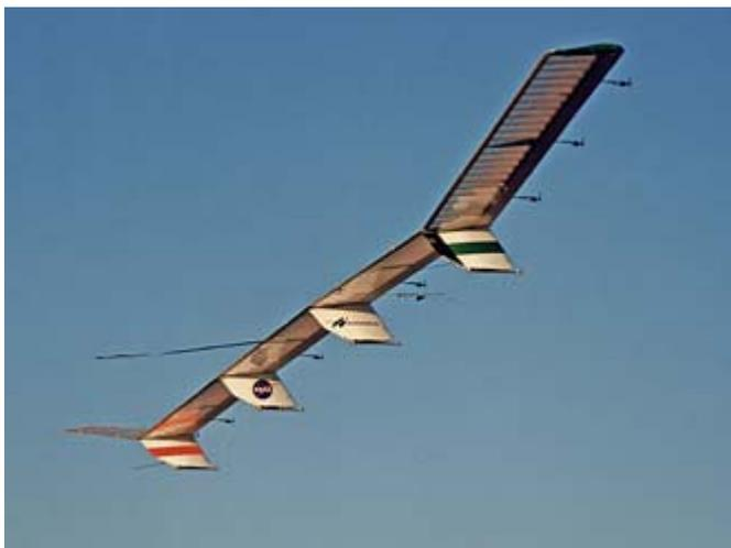
Although it shares much of the design concepts of the Pathfinder, the Centurion has a wingspan of 206 feet, more than twice the 98-foot span of the original Pathfinder and 70 percent longer than the Pathfinder-Plus' 121-foot span. At the same time, it maintains the eight-foot chord (front to rear distance) of the Pathfinder wing, giving the Centurion wing an aspect ratio (length-to-chord) of 26 to 1.
