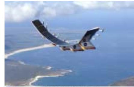
Unmanned Helios Aerovironment 30'000 m, 21 KW
