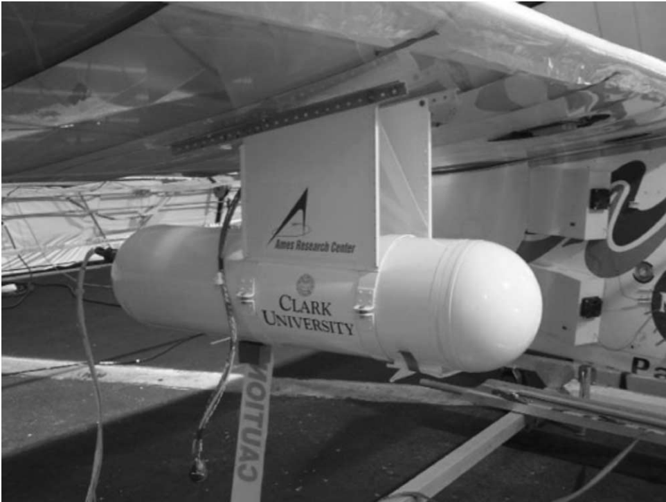
Fig. 2. DuncanTech pod attached to underside of Pathfinder-Plus UAV wing.
