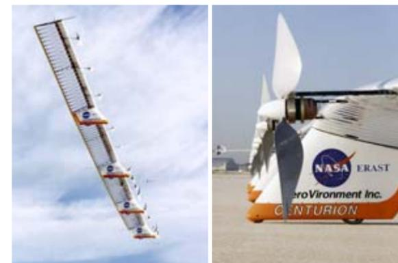
The next step for Centurion was the addition of a 6th wing panel to bring the overall wingspan up to 250 ft. This was being done
