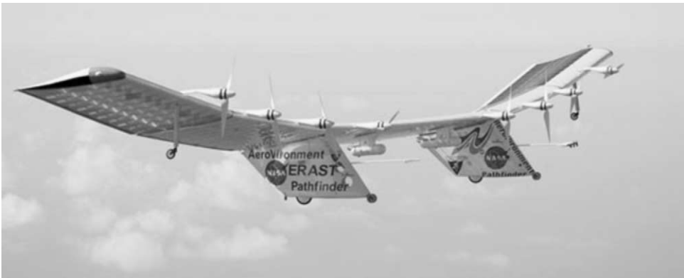
Fig. 3. Pathfinder-Plus UAV in flight over Kauai on 30 September 2002. Cameras are housed in environmental pods suspended near wing center.
