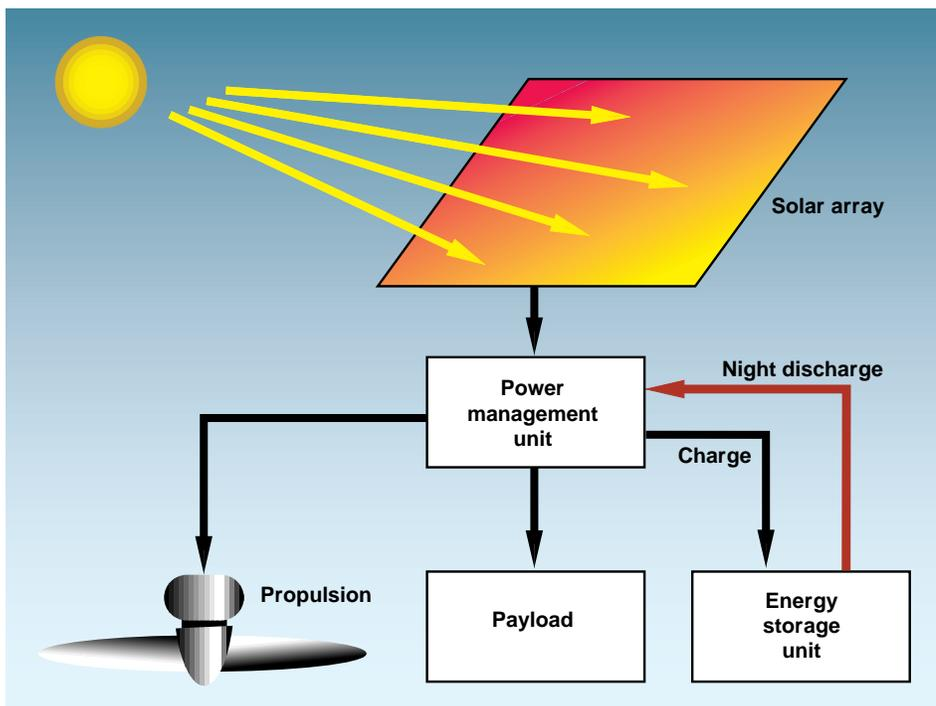
**Figure 1.** A simplified schematic of solar-rechargeable, round-the-clock flight. Less than half the sunlight striking the solar cells powers the motors; a larger fraction is stored on board. As the solar energy striking the cells falls below a certain minimum, the aircraft’s power-management unit begins drawing on the stored energy for the “night” portion of the flight.
