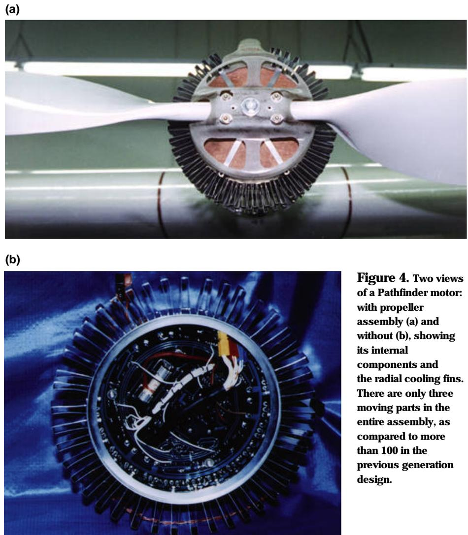
**Figure 4.** Two views of a Pathfinder motor: with propeller assembly (a) and without (b), showing its internal components and the radial cooling fins. There are only three moving parts in the entire assembly, as compared to more than 100 in the previous generation design.
