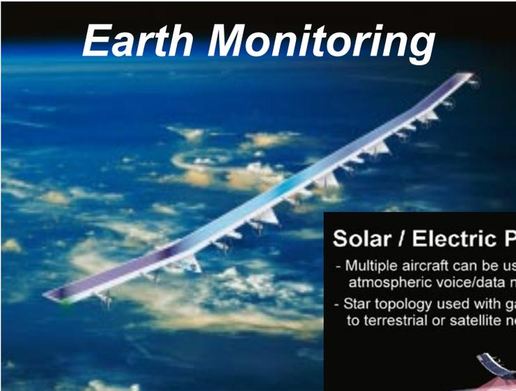
Develop solar aircraft technology to open the door to low cost ultra-long duration high altitude flight.
